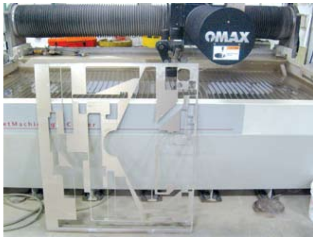
Wagner Machine Co. wanted its Omax 2652 Waterjet cutter to autonest to save time that was spent manually creating part nests in CAD and exporting them. It found a solution with Jetcam Expert. Shown is one of the intricate parts that was manufactured.
